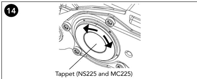
**14** After assembly check that the tappet boot seal assemblies are securely attached by pulling them lightly by hand. Check that the tappets are free to rotate slightly in each direction, taking care not to over-stress the tappet boots.
