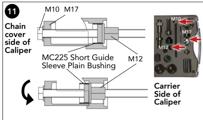
11 To extract the short guide sleeve plain bushing on Webb MC225 models (ref. Webb kit KS0205) use tool combination M10, M12 & M17.
