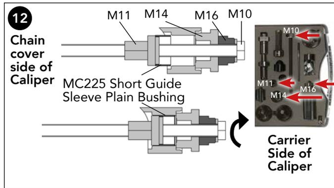
12 To fit a new short guide sleeve plain bushing on Webb MC225 models (ref. Webb kit KS0205) use tool combination M10, M11, M14 & M16. Note that M16 is used as a spacer in order to provide clearance for M10 with the housing.
