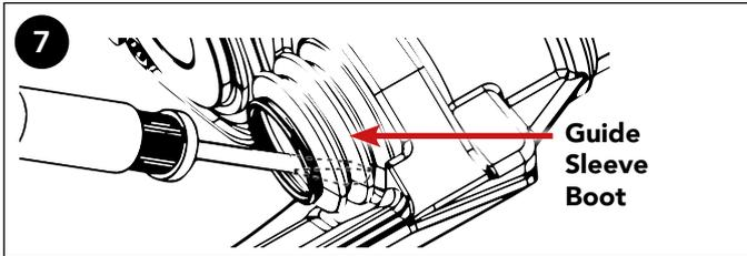
**7** Remove and discard the guide sleeves and plastic washer and ease out guide sleeve boot with a suitable tool (e.g. screwdriver). Check the inside area of the caliper bores and seal interfaces. In case of damage or excessive corrosion the caliper must be replaced.
