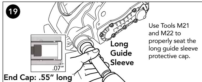
19 Insert the protective cap for the long guide sleeve into the caliper bore – protective cap and bore must be clean and free from lubrication. Press the metal protective cap into the long guide sleeve bore ensuring it is seated squarely until the cap is flush with the cast boss.
