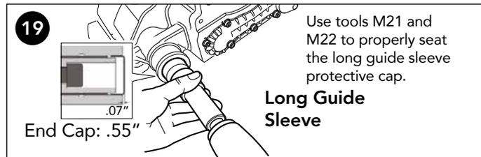
**19** Insert the protective cap for the long guide sleeve into the caliper bore – protective cap and bore must be
