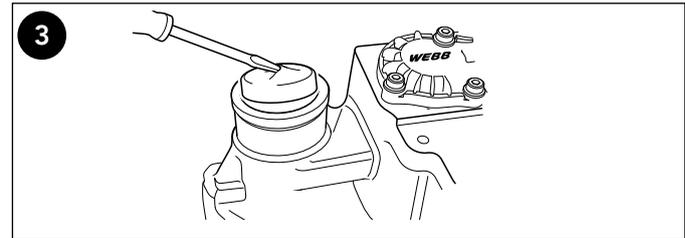
**3** Remove the guide sleeve protective cap by inserting a suitable tool into the created hole and levering it out.
