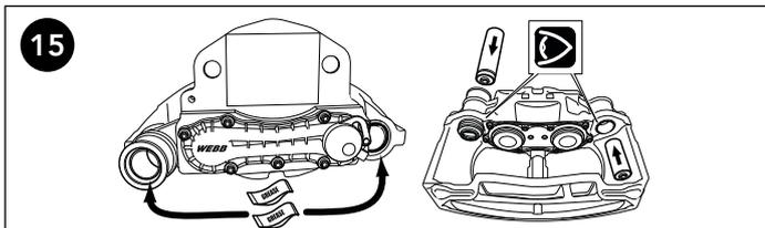
**15** Grease both guide sleeves using the grease packets provided. Slide the guide sleeves into the brass bushing in the directions indicated above
