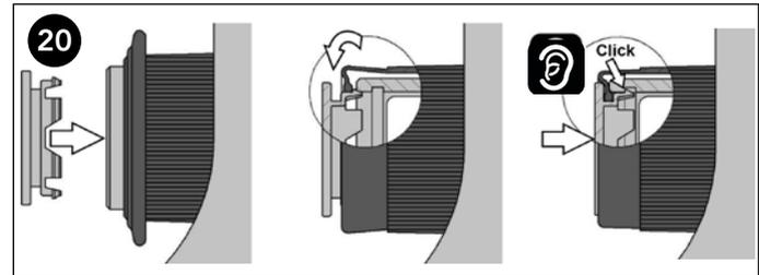
**20** Stretch the rubber bushing bellows over the short guide sleeve and position the plastic cap in the end of the guide sleeve bore – do not push into the bore yet. Slide the bellows back over the plastic cap, ensuring it locates correctly all around the groove, and then push the cap firmly into the guide sleeve so that it clicks into place.
