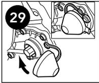
29 Check for free rotation of the disc. Refit the adjuster cap.
