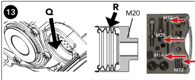
**13** To fit a new guide sleeve boot (ref. Webb Kit KS0200/ KS0205/KS0215) for the long guide sleeve use tool combination M10, M14 & M20. The assembly process for the guide sleeve boot for the short guide sleeve (for Webb Kit KS0205) is the same method as for the long guide sleeve **but for MC225 short guide sleeve boot add tool M13 between M10 and M14** to act as a spacer (MC225 has 2 boots and the spacer is not required for the long guide sleeve boot).
