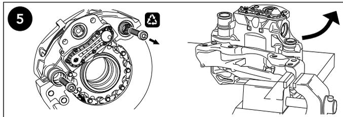
**5** Remove and discard the guide sleeve bolts and remove the caliper from the carrier. If the brake is removed from the vehicle ensure the carrier is securely located to resist the bolt torque, at a location close to the bolt being tightened, to prevent damaging the carrier.
