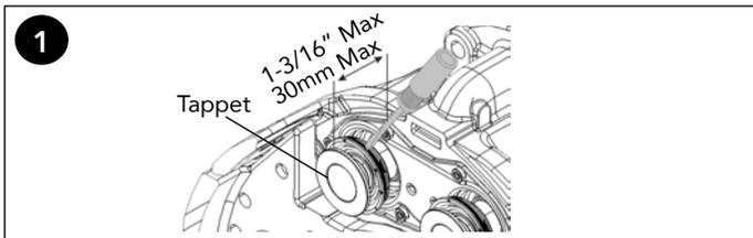
**1** Remove the brake pads. Adjust the tappets forwards using a 10mm socket or wrench on the adjuster (do not exceed 18.5 ft-lb torque) until the tappet boots are easily accessible. The tappets must not be extended more than 1-3/16" (30mm) from the caliper face to ensure the pistons remain synchronized. With a suitable lever (e.g. screwdriver) carefully pry the tappet boot out. Take care not to damage the sealing surface on the caliper cover plate.
