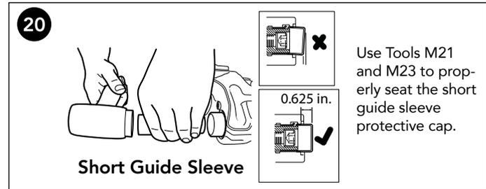
20 Insert the protective cap for the short guide sleeve into the caliper bore – protective cap and bore must be clean and free from lubrication. Press the protective cap into the bore until the cap protrudes .625" from the cast boss, ensuring it is seated squarely.
