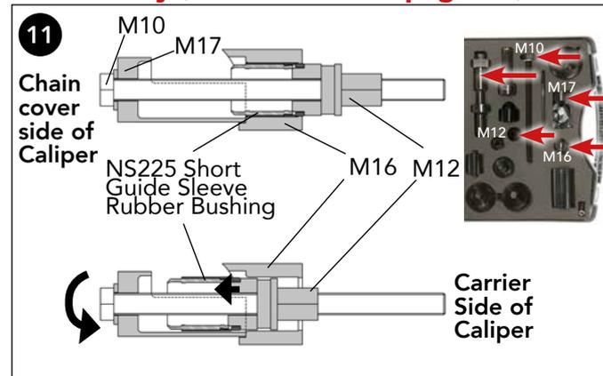
11 To extract the short guide sleeve rubber bushing (ref. Webb kit KS0200/KS0215) use tool combination M10, M12, M16 & M17 from the Webb caliper service
