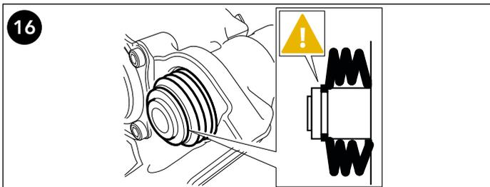
**16** Insert the boots into the sealing groove in the guide sleeves ensuring they seal correctly all around the sleeves.
