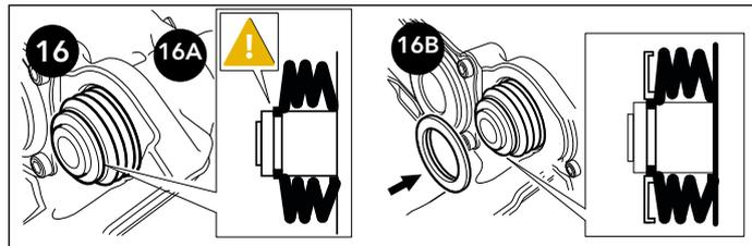
**16a** Insert the boot into the sealing groove in the long guide sleeve ensuring it seals correctly all around the sleeve.
