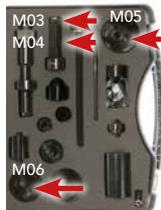
fitment on the vehicle, adding tool M04 (between M03 & M05) if the brake is removed from the vehicle. Tool M07 in Webb Caliper Service Tool Kit KS0010 is not required for Webb calipers.
