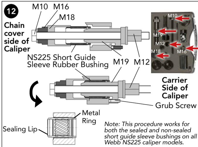
**12** To fit a new NS225 short guide sleeve rubber bushing (ref. Webb kit KS0200/KS0215) use tool combination M10, M12, M16, M18 & M19. The grub screw on M19 should be wound in so that it does not contact the caliper surface, and M19 is aligned with the guide sleeve bore.
