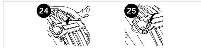
**24** Insert the new pad retainer in the slot in the caliper and depress to enable the insertion of the pad retainer pin. Position the washer over the pad retainer pin.
