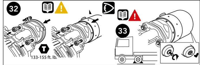
32 Reinstall the air chamber in the same orientation as when removed, in accordance with the vehicle manufacturer's recommendations. Tighten the nuts to 133-155 ft. lb. (unless specified differently in the vehicle manufacturer's recommendations).
