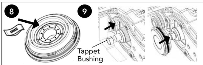
**8** Clean and check the **cover plate sealing face** and the **threaded pistons for damage or corrosion** – these cannot be replaced and if damaged the caliper must be replaced. Lubricate the inner abutment face of both tappet heads with BLACK grease (ref. KA1505) being careful not to transfer the grease to other components.
