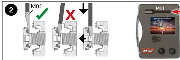
**2** Position the forked wedge tool (M01) between the threaded piston and the tappet boot seal assembly with the stepped side towards the tappet boot. Carefully drive it down with a hammer to release the tappet boot seal assembly from the threaded piston. Keep the tool perpendicular to the piston – do not lever the tappet or damage the piston thread.
