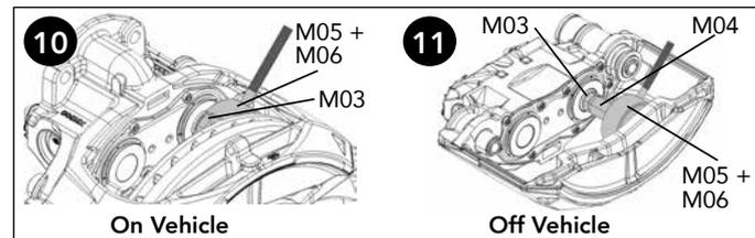
**10** If **on vehicle** position tool combination M03, M05 & M06 so that the closed side of M06 touches the brake disc. Wind out M03 using a wrench to press the tappet boot seal assembly until it stops.
