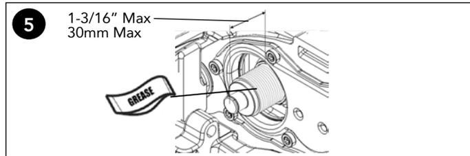
**5** Wind out the threaded pistons using a 10mm socket or wrench (do not exceed 18 ft-lb torque) to a maximum extension of 1-3/16" (30mm). Check the pistons for damage or corrosion. If there are signs of water ingress beyond the inner boots the caliper must be replaced.
