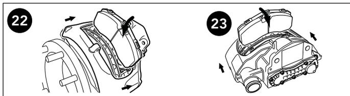
**22** Slide caliper inboard and insert inner brake pad and spring.
