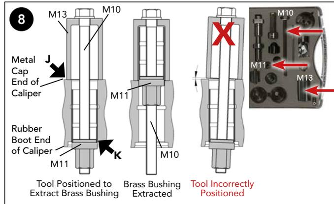
**8** To extract the long guide sleeve brass bushing, use tool combination M10, M11 & M13 from the Webb Caliper Service Tool Kit (ref. KS0010 or equivalent).
