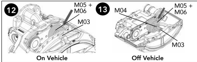
**12** If **on vehicle** release the tool and turn tool M06 over, within M05, so that the open side of M06 makes contact with the tappet boot seal. Ensure it is centered on the tappet.
