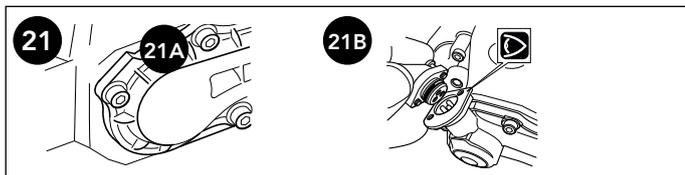
**21** If the carrier was removed from the vehicle, reinstall the caliper and carrier assembly in accordance with the vehicle manufacturer's recommendations. Reconnect the pad wear sensor cable connector (where applicable).
