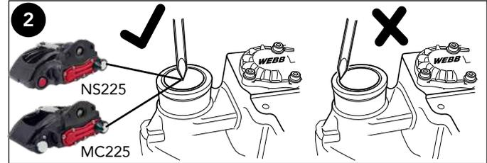
**2** Pierce the middle of the protective cap on long guide sleeve using a suitable tool. Do not drive the tool between caliper bore and cap, as this might damage the caliper bore.
