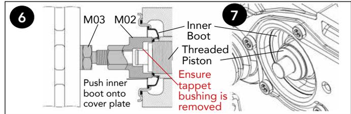
**6** Ensure that the old tappet bushing is removed. Position tool combination M02 & M03 over the boss of the threaded piston and wind out until M03 touches the brake disc. **If the caliper is removed from the vehicle add tool M04 (between M02 & M03)** and wind out until M03 touches the outboard pad abutment face of the caliper.
