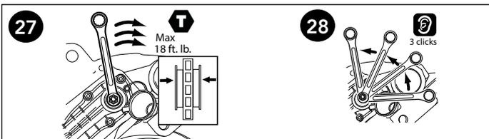
**27** Turn the adjuster clockwise until the pads come into contact with the disc - do not exceed 18 ft. lb. torque.
