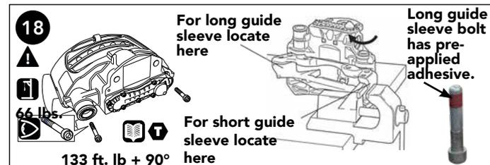
**18** Ensure the carrier threads are clean, dry and free of lubrication and/or residuals of pre-applied adhesive (the
