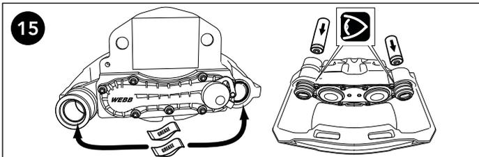
**15** Grease both guide sleeves using the grease packets provided. Slide the guide sleeves in to the bushings in the directions indicated above.
