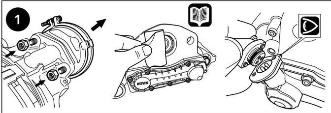
**1** Remove the brake pads and air chamber from the caliper in line with the vehicle manufacturer's recommendations.
