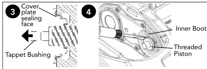
**3** Remove the tappet bushing from the end of the threaded piston. Clean and check the cover plate sealing face and the threaded pistons for damage or corrosion. **The pistons and cover plate cannot be replaced and if damaged the caliper should be replaced.**
