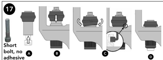
**17** **A** Fit the short bolt into the guide sleeve with pre-assembled rubber boot in the direction indicated.
