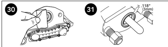
30 Remove the adhesive tape in the area of the air chamber attachment. Take care that no dirt enters the brake caliper.
