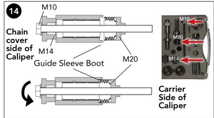
**14** Assemble the prepared parts, with the new guide sleeve boot fitted into M20, through the caliper bore from opposite ends and screw M20 onto M10 by hand until it stops. Take care not to tilt the guide sleeve boot when winding it in.
