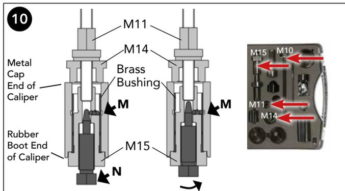
10 To prevent axial movement of the brass bushing it must be "staked" into the bore (arrow M). The hexagonal bolt of tool M15 (arrow N) must be screwed in up to its stop to deform the brass bushing into place.
