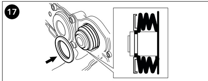
**17** Position the plastic washer over the boots to retain them in the sealing groove in the guide sleeves. Ensure that the washer is in the correct orientation.
