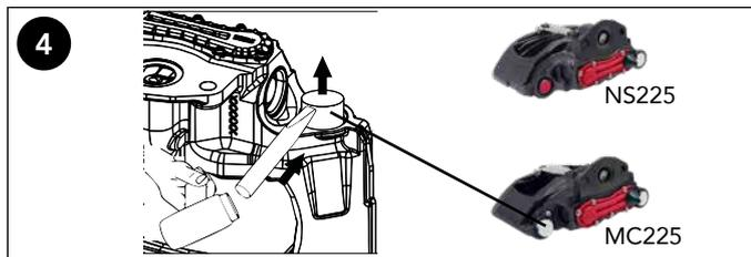
**4** The longer protective cap covering short guide sleeve (MC225 models) should be removed from the side and in an upward direction. Do not hit the protective cap in the direction of the caliper as this might damage the caliper. For NS225 models with a sealed short guide sleeve, gently pry out the plastic guide sleeve end cap using a flat head screwdriver.
